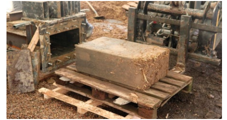
Block in 1:4 scale pressed from recycled cob mass from a Thuringian building dating 1711 during a pilot test. Photo Ute Reeh
